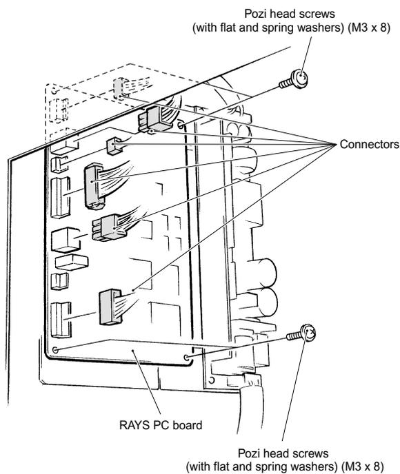
3. Remove 4 off pozi head screws (M3x8), with flat and spring washers, and remove the RAYS PCB.
