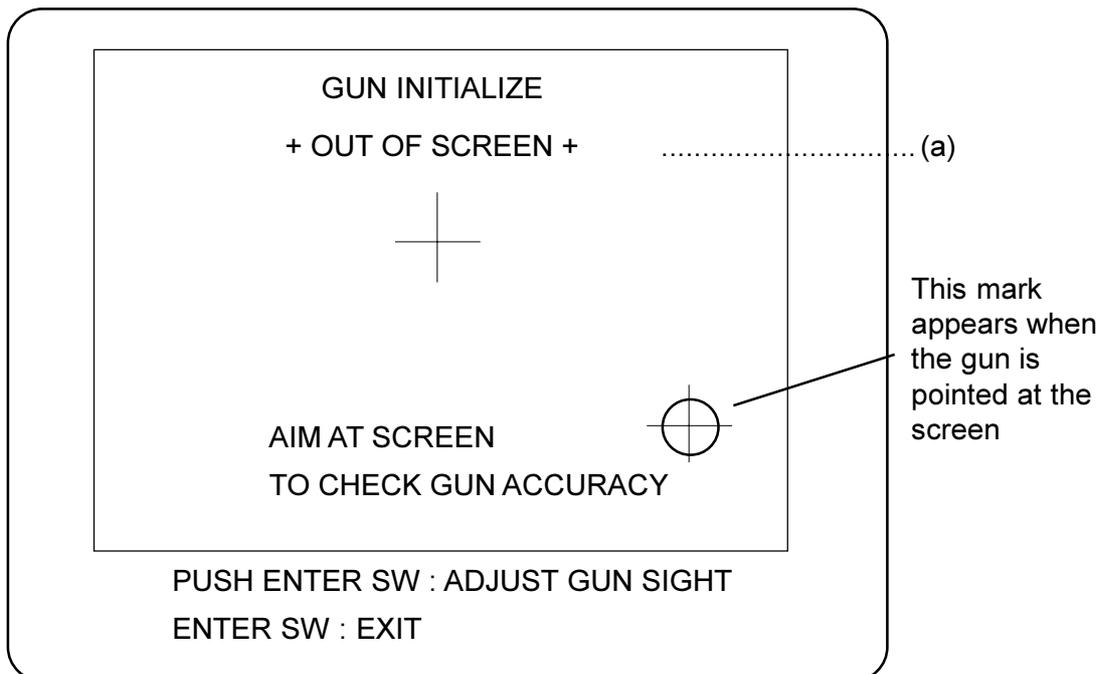
2. When the gun is pointed at the screen, a cross appears at the point where the gun is aimed. Check that the gun sight and cross are aligned. (Make sure that the gun can aim at areas near the edge of the screen). When the gun is pointed away from the screen, "+OUT OF SCREEN +" appears on the screen (item a).
