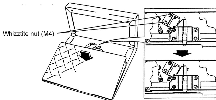
4. Refit the switch cover plate and 4 off security screw (M5x12).
