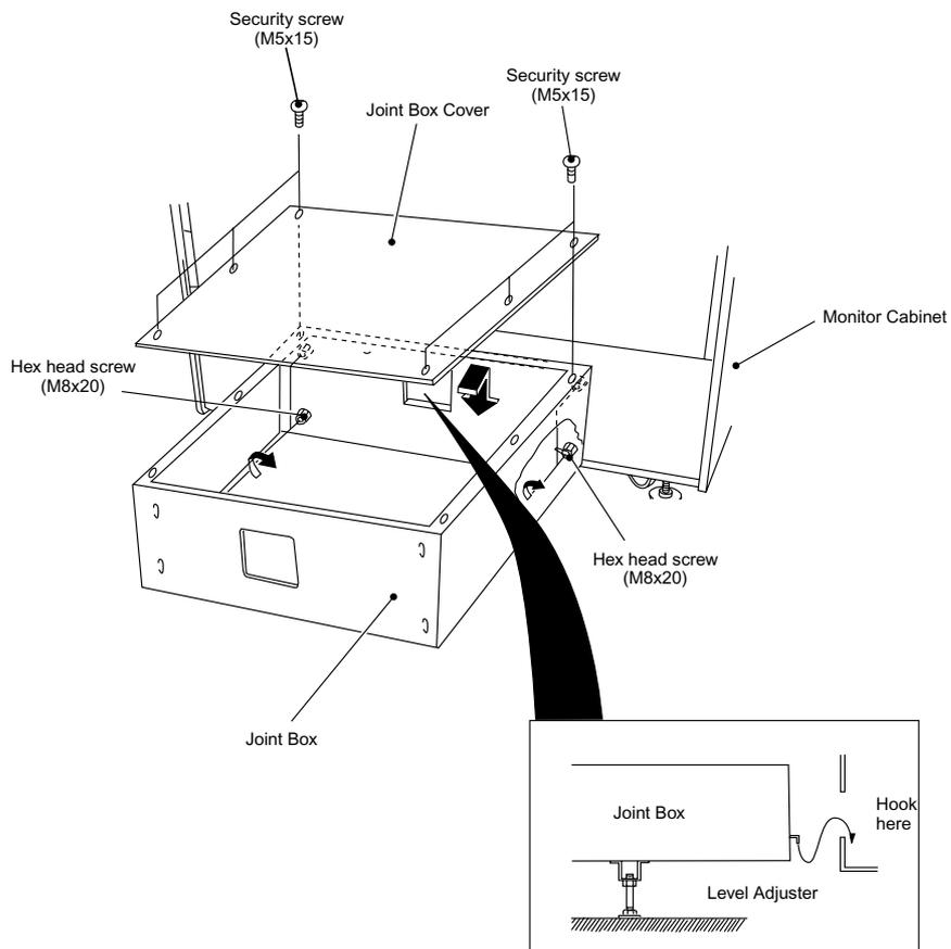
3. Fit the hook of the Joint Box into the Hole on the Projector Base and fit, finger tight only, 4 off hex head screws (M8x20) to retain the Joint Box to the Monitor Cabinet.
