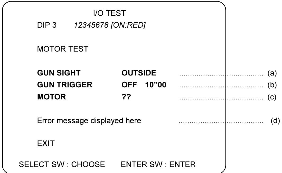
2. The gun motor will operate when the trigger pulled. When the gun is pointed at the screen, "INSIDE" is displayed next to 'GUN SIGHT' (item a). When the gun is pointed away from the screen, "OUTSIDE" is displayed next to 'GUN SIGHT' (item a). *If these indications do not appear properly, adjust the Gun Sight (see section 5-2-3-2 page 52) before checking the Gun Motor.*
