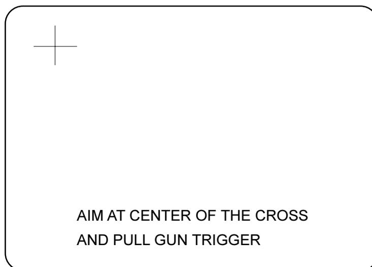
6. Aim the gun at the cross mark in the upper left corner of the screen, and pull the trigger. After the trigger is pulled the screen will advance to the next step.
