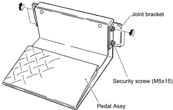
2. Connect the connectors between the Pedal Assy and the Cabinet.
