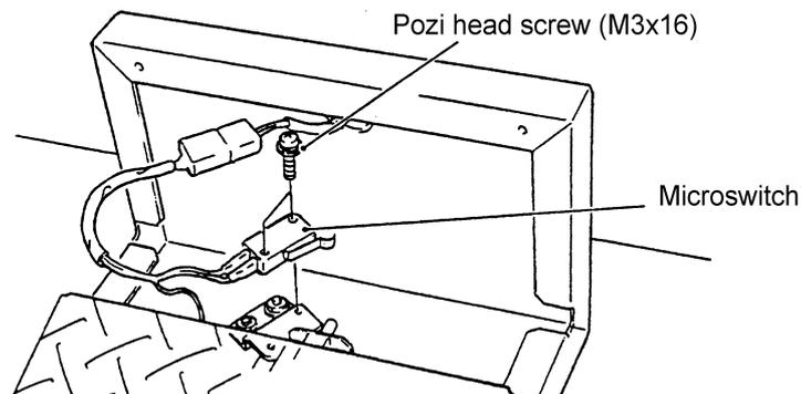
3. Slacken the 2 off whizztite nuts (M4) and adjust the microswitch bracket so that the switch plunger operates the switch correctly without bending the switch lever against the switch body.
