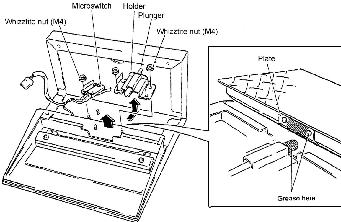
5. Grease both the plate and spherical portion of the plunger.
