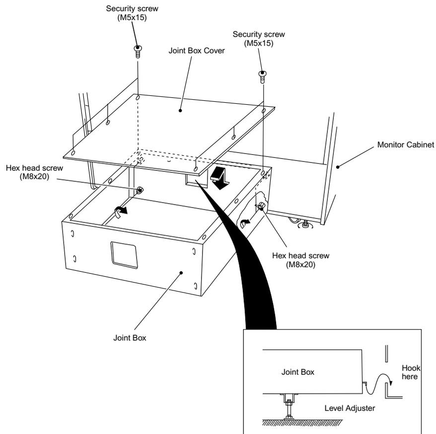
6. Fully tighten the 4 off hex head screws (M8x20).
