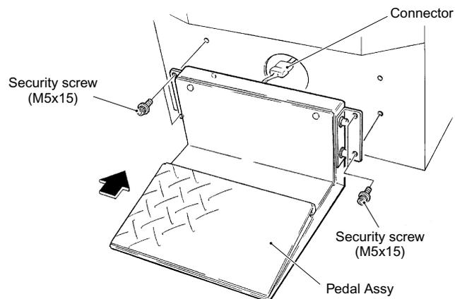
6. Ensure that the Pedal Assy is flat on the floor and fully tighten the 8 off security screws (M5x15)
